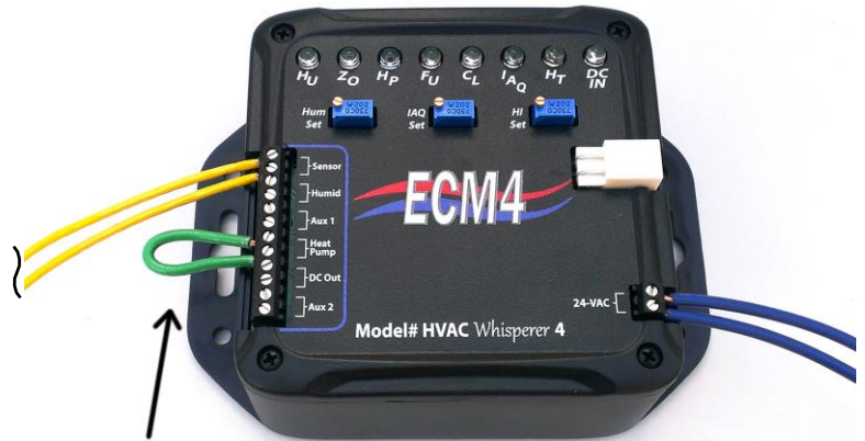
Place Jumper between terminals 7&8
